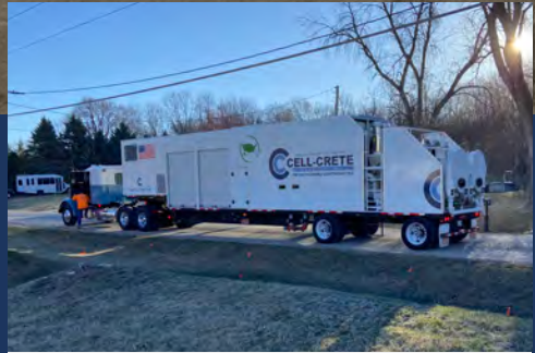
Colloidal Hydraulic Mixer (Dry Mix) – Provides high-shear mixing for consistency.
